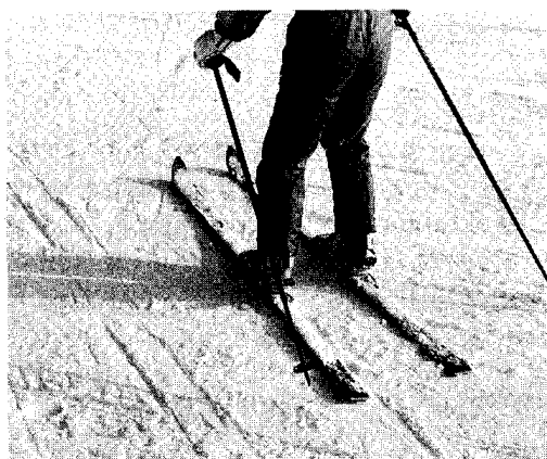
Fig. 5. Observing the shadow of the skis, edging angle \beta of the left leg against the snow surface appears larger than that of the right leg. This figure corresponds to Fig. 3(c) and the case of ski number 1 in Fig. 4.
