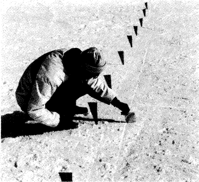
Fig. 5. The author (Sahashi) measuring the angle \beta_0 on a plane of a sliding track.
