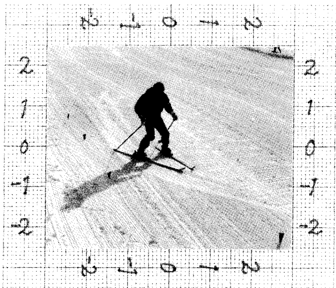
Fig. 8. Method of reading coordinates of the skis from the photograph. Skier: Ichino, at Hoonoki-daira Ski Resort, taken on February 4, 1994.
