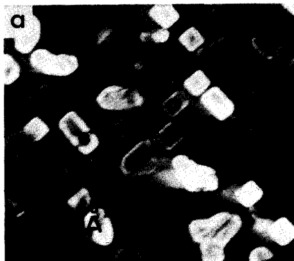
Fig. 4. Dark field images at 100 kV. (a) (200) reflection. (b) (220) reflection.
