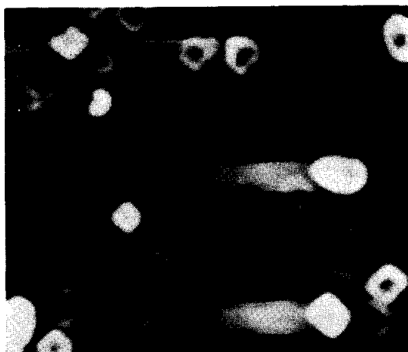
Fig. 3. Dark field image at 50 kV, (200) reflection.
